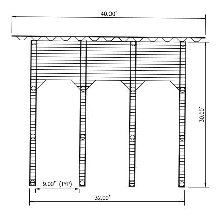
A vinyl sheet pile bulkhead will be constructed in the location of the existing deteriorated wall. The boat house/deck will be constructed adjacent to the new bulkhead. Old pilings and wood decking will be replaced with treated timber piles and decking. Roofing will be 26 guage metal roofing.
